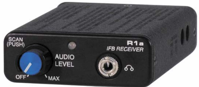
Figure 1 - R1a Control Panel
