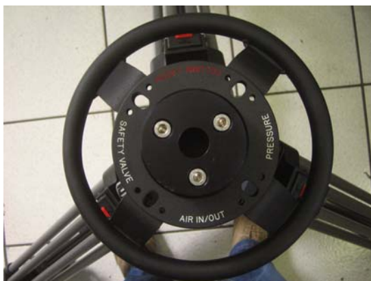
Figure 4 — Air in/out, safety valve and pressure gauge
