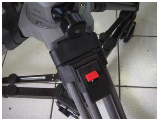
Figure 4 — Tripod lever for height adjustment
