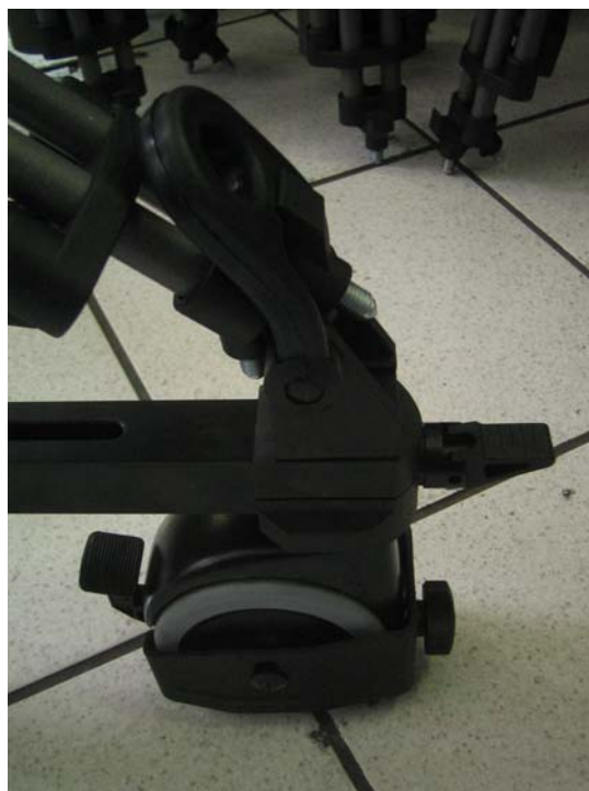
Figure 10 — Hook for tripod locking and wheels position locking levers
