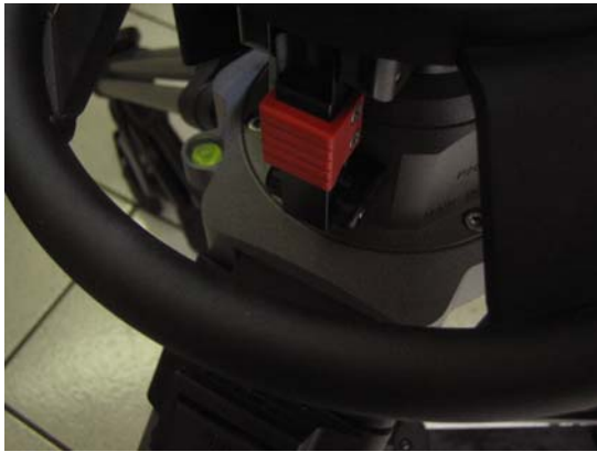
Figure 6 – Column sliding locking lever
