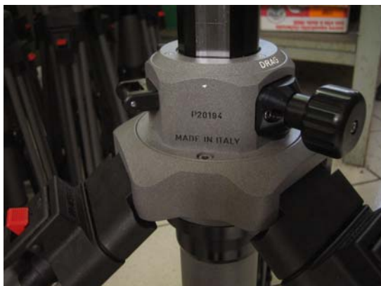
Figure 9 — Potential risk of fingers being trapped and Drag and Lock knobs
